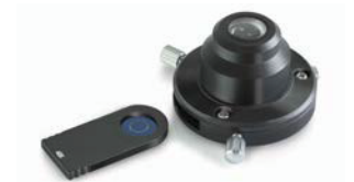
Simple PH condenser with 40x PH slide
